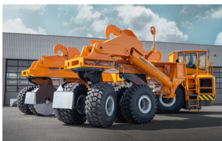
The KAMAG SPC (Slag Pot Carrier) for safe and reliable slag handling – developed for demanding operating conditions and optimized for current requirements in steel production. A record-breaking 170-ton version has recently been delivered to a customer operating an Electric Arc Furnace.
