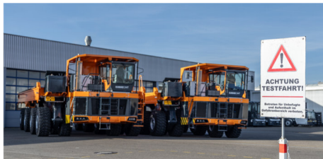
The KAMAG IHT (Industrial Heavy Transporter) – designed for efficient in-plant heavy-duty transport and increasing demands in modern steel production processes.
