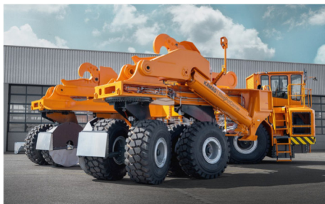
The KAMAG SPC (Slag Pot Carrier) for safe and reliable slag handling – developed for demanding operating conditions and optimised for current requirements in steel production. A record-breaking 170-tonne version has recently been delivered to a customer operating an Electric Arc Furnace.
