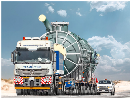
International project deployment in Saudi Arabia: Teamlifting transports a large-scale industrial component on modular SCHEUERLE K25 axle modules
