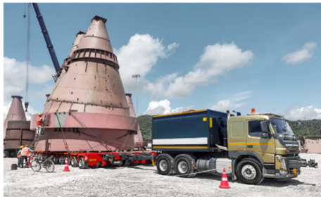
Heavy transport project in India: iRISE moves a large-scale industrial component using modular SCHEUERLE K25 axle modules.
