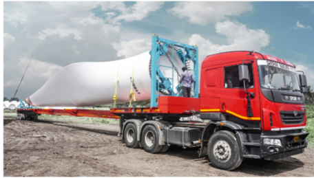
SCHEUERLE Extender units from the Bawal site: The vehicles are used for the transport of rotor blades.
