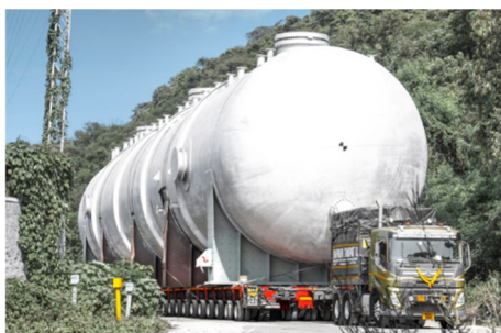
Project transport in India: Bhagyodaya Transport Limited. moves a process vessel weighing approximately 450 tons for Fabtech on modular SCHEUERLE K25 axle modules.
