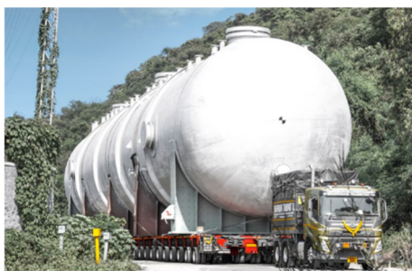
Project transport in India: Bhagyodaya Transport Limited. moves a process vessel weighing approximately 450 tonnes for Fabtech on modular SCHEUERLE K25 axle modules.
