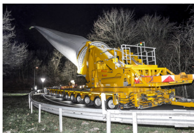
This means rotor blades can be swivelled over obstacles such as buildings and carriageway dividers...
