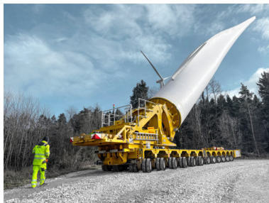
This rotor blade measures 84 metres long. The set-up angle of 60° provides the best possible manoeuvrability.
