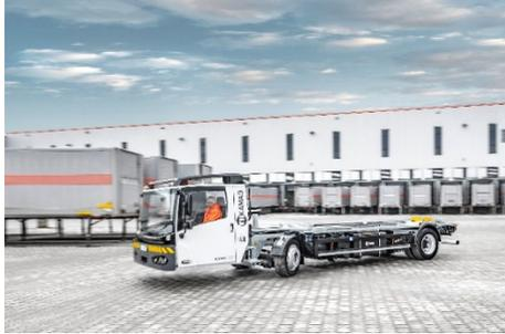
The hot-dip galvanised version of the KAMAG PM in use at the depot.
