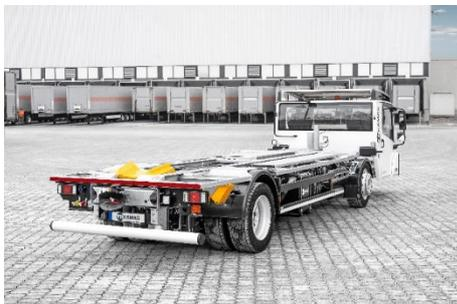
The galvanised frame, lifting table and cab mounting system provides the KAMAG PM with reliable corrosion protection.
