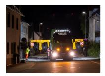
Robust axle lines: 18 SCHEUERLE InterCombi axle lines supported the successful transport. Each of the two convoys had a total weight of 250 tons and altogether an overall length of 50 meters. Kübler mastered all bottlenecks with flying colors.
