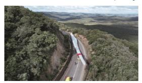
Vanguard is currently transporting more than 230 rotor blades for 78 wind farms to the inland installation sites 500 km away using RBTS systems from TII SCHEUERLE.
