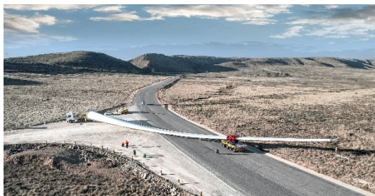
SCHEUERLE RBTS (Rotor Blade Transport System) with an 83 metre long rotor blade.
