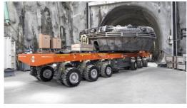
Further challenges followed when transporting tunnel boring machine parts in a very confined space. After this, the 4 SCHEUERLE SPMT PowerHoss units are now being used as gantry crane chassis tasked with transporting concrete slabs at Geneva Airport.
