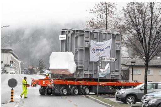
Flexible route selection: Firstly, Friderici Spécial transported two transformers weighing 100 and 147 tonnes respectively.
