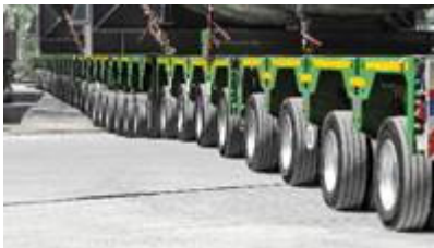
A total of 30 SCHEUERLE InterCombi axle lines were required to evenly distribute the load and thus fully protect the forest floor of the nature reserve.
