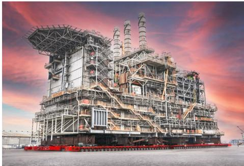
The introduction of SCHEUERLE SPMT technology revolutionized production. Since then, it has been possible to transport even gigantic components up to complete industrial and conveyor systems. Pictured: a 14,300-ton oil and gas platform.
