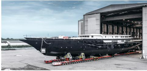
Roll-out of the 127-meter luxury yacht on a SCHEUERLE SPMT. SCHEUERLE SPMTs are also widely in use in shipyards. Shown in the photo: *Koro*, the latest luxury yacht from Jeff Bezos.
