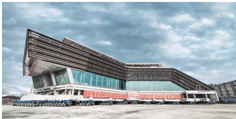
The modularity and combinability of SCHEUERLE SPMT axle lines allow the number of axle lines to be flexibly adapted to the respective payload requirement. This enables customers to successfully undertake spectacular projects. Shown in the photo: a 7,500-ton hotel in China was moved 500 meters on SCHEUERLE SPMT due to environmental protection requirements.
