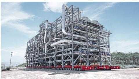
With the introduction of the SCHEUERLE SPMT in 2,430 mm width, transport undertakings could now take place even in the most remote places in the world. The container width enables fast, efficient, and more cost-effective transport of the SCHEUERLE SPMT modules in flat-rack containers.
