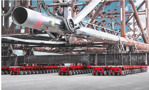
Whether coupled together or in an open network - there are no limits to the possible combinations of SCHEUERLE SPMTs. Thus, the payload is theoretically unlimited.
