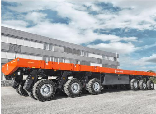
Extension of the series through the SPMT PowerHoss 330 with 6 axle lines and a 330-tonne payload.
