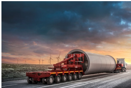
A combination featuring the K25L and WT70 - for wind tower segments of the most powerful wind turbines.
