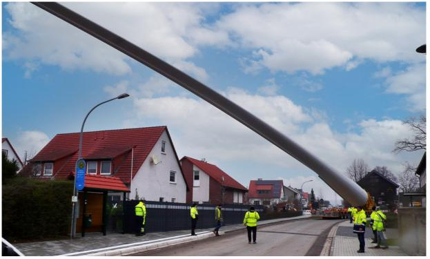
Successful transport: with the SCHEUERLE InterCombi, approx. 80 metre long rotor blades were transported to the Flöthe wind farm. Through the help of the rotor blade adapter G4, wind blades of up to 900 metre tonnes can be lifted up to 60° and thus safely negotiate every bottleneck and swivel over numerous obstacles.
